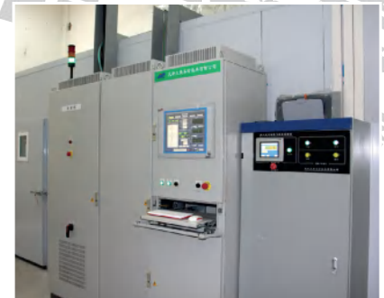
12. Rolling Resistance Testing Machine
