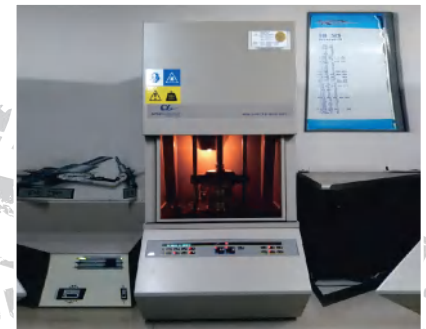
10. ALPHA Curemeter Without Rotator
