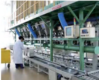
1. Automatic chemical powder weighing system for mixer
