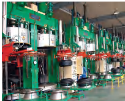
6. Steel-belted radial tyre hydraulic dual-mould curing press
