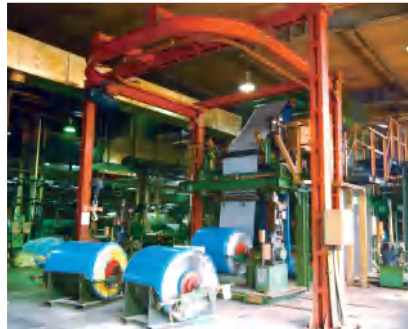
2. Steel cord calendar made by Comerio Ercole of Italy
